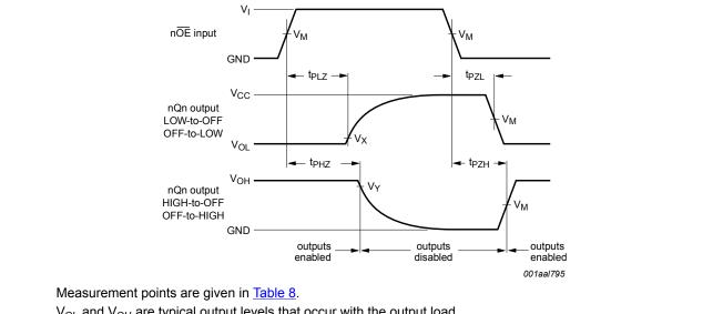
$V_{OL}$  and  $V_{OH}$  are typical output levels that occur with the output load.
