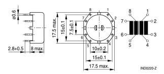
Tolerances to ISO 2768-M unless otherwise noted. Dimensions in mm.
