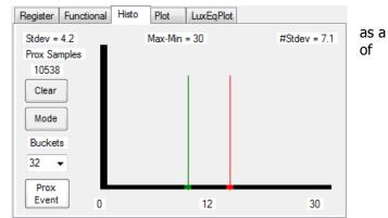
The three numbers below the Horizontal axis show the minimum value, maximum value, and mean of the displayed samples. The red vertical line shows the proximity detection threshold as set by the sliders on the input side of the GUI.
