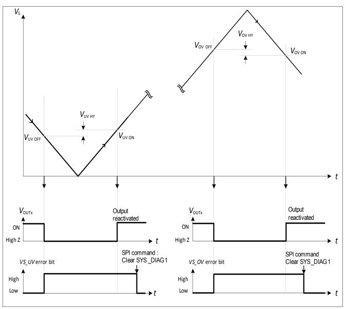
Figure 12 Output behavior during under- and overvoltage V<sub>s</sub> condition
