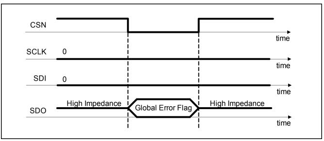
Figure 16 SDO behaviour with 0-clock cycle
