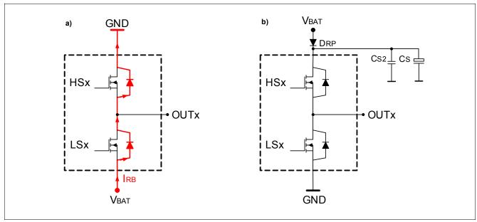
Figure 4 Reverse Polarity Protection
