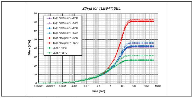
Figure 29 ZthJA Curve for different PCB setups
