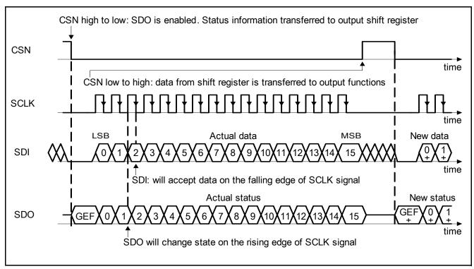
Figure 13 SPI Data Transfer Timing (note the reversed order of LSB and MSB as shown in this figure compared to the register description)
