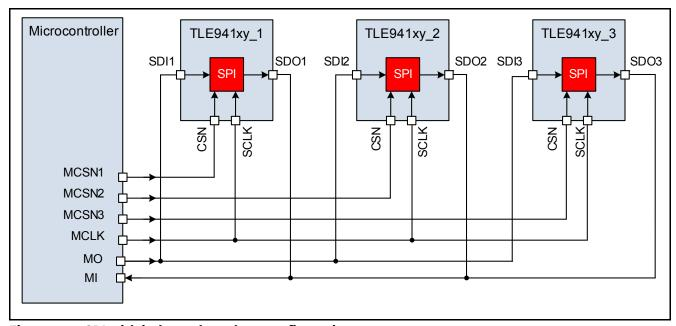
Figure 18 SPI with independent slave configuration
