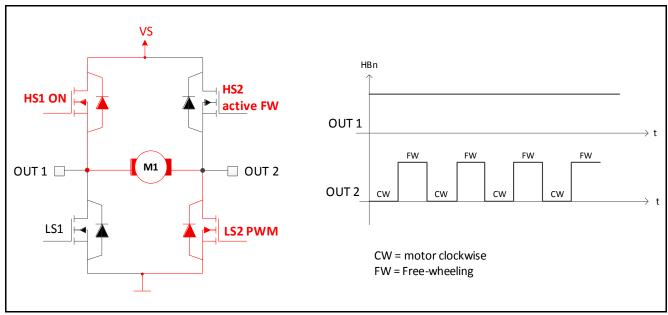
Figure 5 PWM operation on OUT 2
