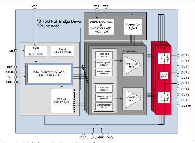
Figure 2 Block Diagram TLE94110EL (SPI Interface)
