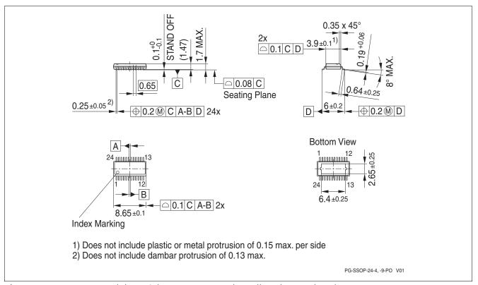
Figure 31 PG-SSOP-24 (Plastic/Plastic Green - Dual Small Outline Package)
