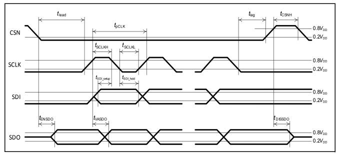
Figure 15 SPI Data Timing
