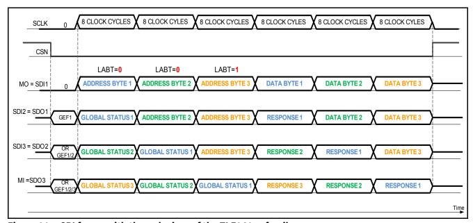
Figure 21 SPI frame with three devices of the TLE941xy family
