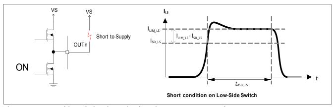
Figure 8 Low-Side Switch - Short Circuit and Overcurrent Protection
