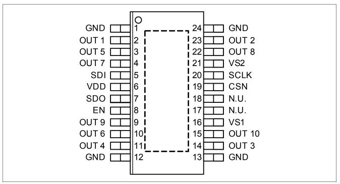
Figure 1 Pin Configuration TLE94110EL
