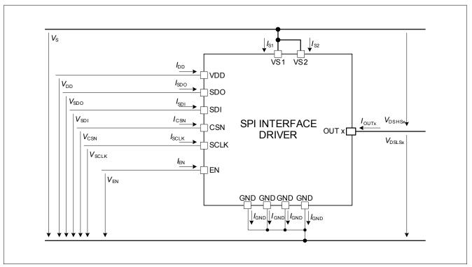
Figure 3 Voltage and Current Definition
