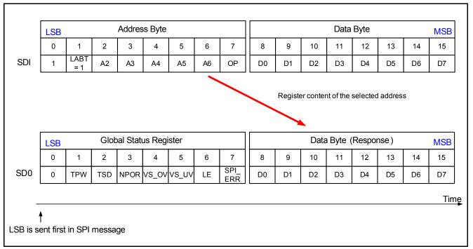
Figure 19 SPI Operation Mode with independent slave configuration
