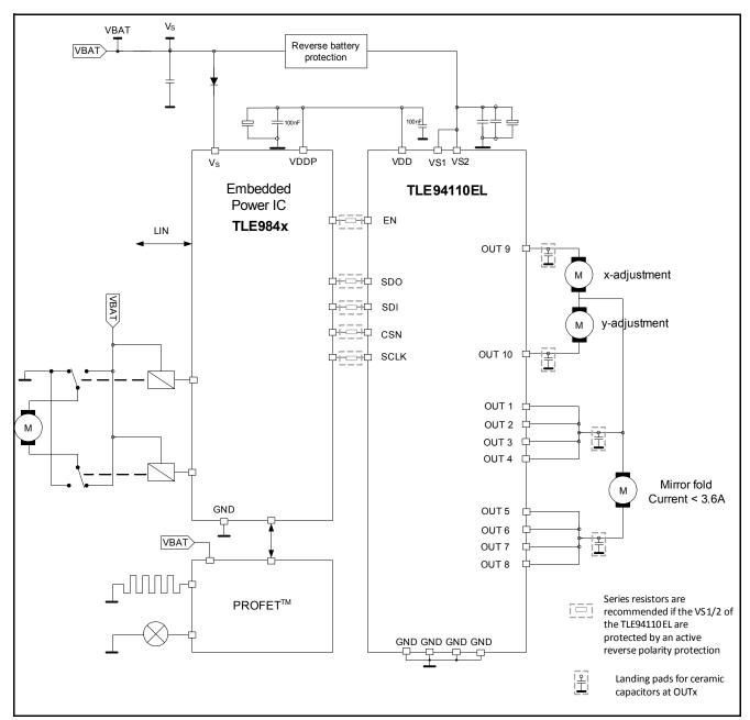
Figure 28 Application example for side-mirror control
