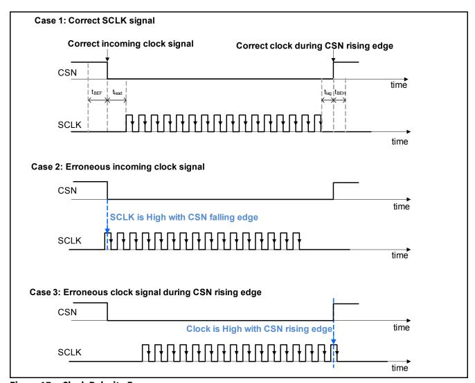
Figure 17 Clock Polarity Error
