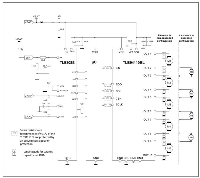
Figure 27 Application example for DC-motor loads
