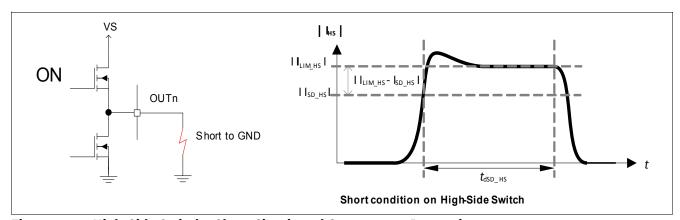
Figure 7 High-Side Switch - Short Circuit and Overcurrent Protection
