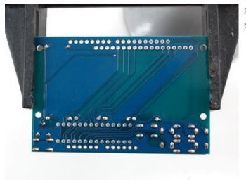
Flip over the PCB and solder in the three legs of the potentiometer and then all 28 pins of the port expander.
