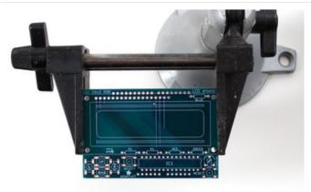
Put the printed circuit board into a vise or board holder, heat up your soldering iron and make sure you're ready to go!
