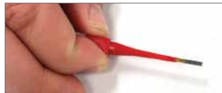
Plastic tool with contact in proper position.
