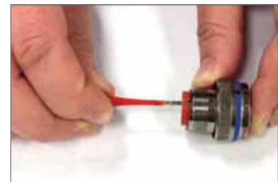
Plastic tool with contact in proper position.
