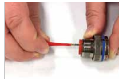
Plastic tool with contact in proper position.
