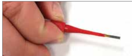
Plastic tool with contact in proper position.
