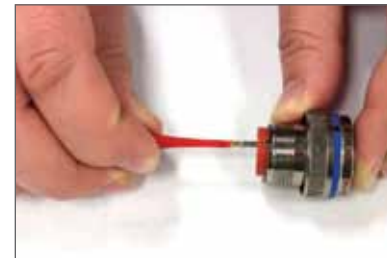
Plastic tool with contact in proper position.
