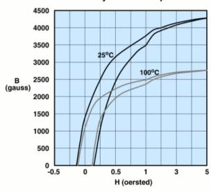
Measured on a 17/10/6mm toroid at 10kHz.
