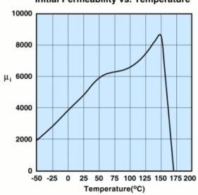
Measured on a 17/10/6mm toroid at 10kHz.
