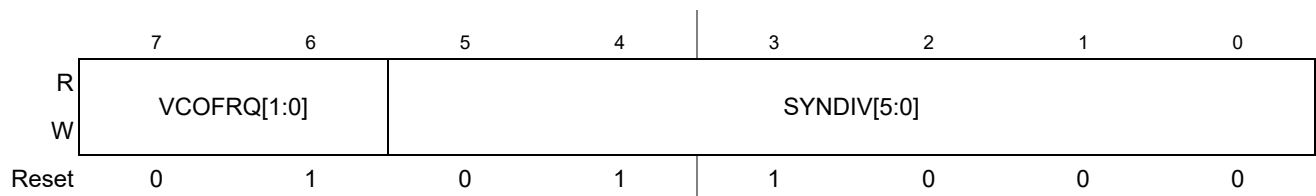
Figure 8-7. S12CPMU_UHV_V11 Synthesizer Register (CPMUSYNR)
