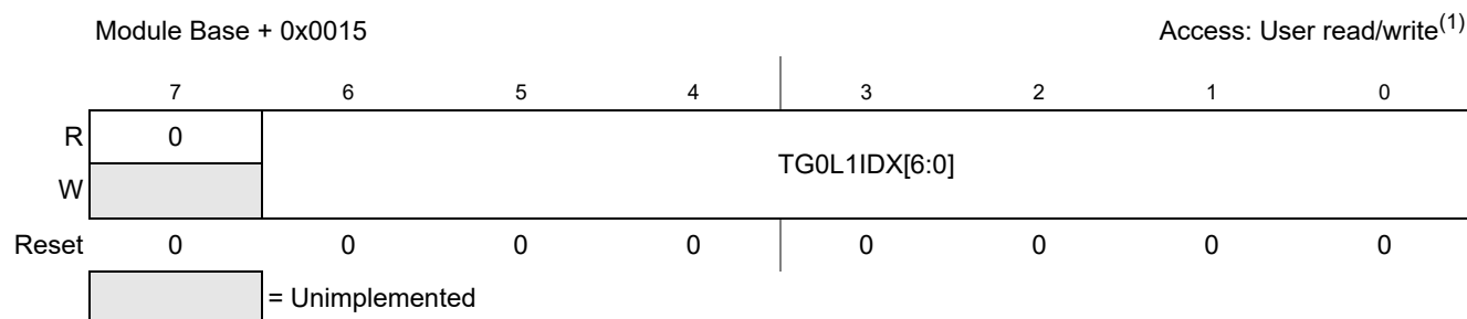
Figure 13-15. Trigger Generator 0 List 1 Index (TG0L1IDX)
