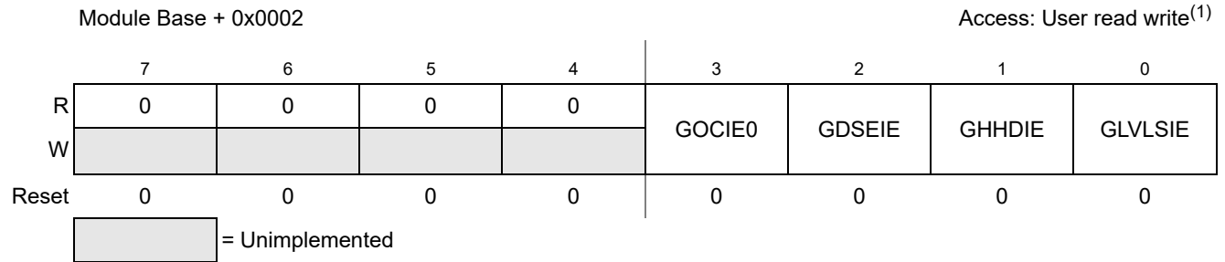
Figure 17-5. GDU1PHV1 Interrupt Enable Register (GDUIE)
