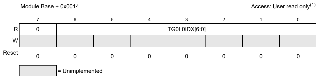
Figure 13-14. Trigger Generator 0 List 0 Index (TG0L0IDX)
