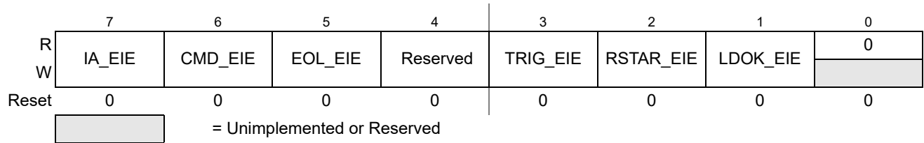
Figure 9-10. ADC Error Interrupt Enable Register (ADCEIE)
