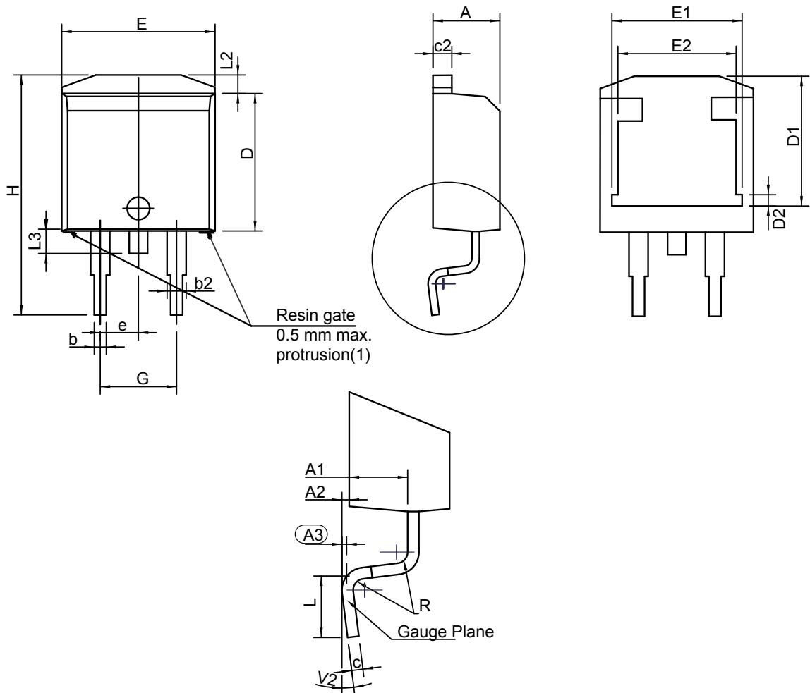
(1) Resin gate position accepted in one of the two positions or in the symmetrical opposites
