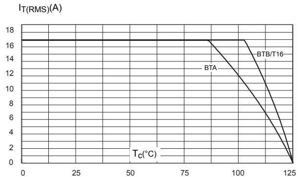
**Figure 4. On-state rms current versus ambient temperature (full cycle)**
