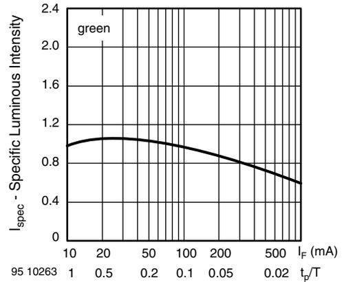
Fig. 6 - Specific Luminous Intensity vs. Forward Current
