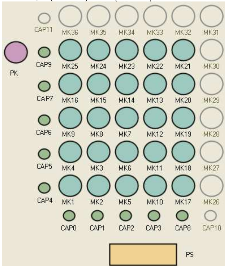
Figure 29: Sensor Status for SX8663 (both PS and PK Enabled)
