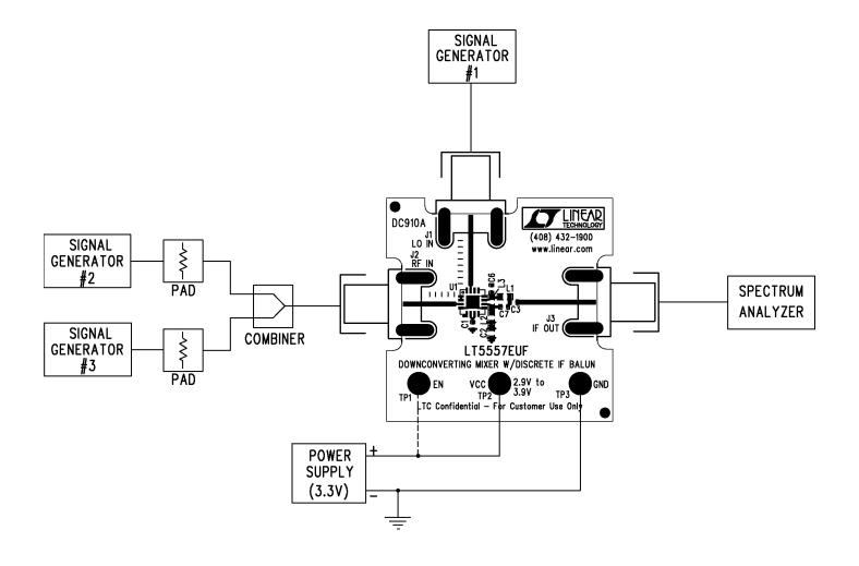
Figure 1. Proper Measurement Equipment Setup
