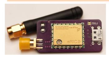
Utilising proprietary LPRS 'easyRadio' technology operating in the 434MHz or 868/915MHz Industrial Scientific & Medical (ISM) bands a pair of eRIC USB 'dongles' can provide a simple 'wireless bridge' between any host devices that support USB serial communications such as a PC or Raspberry Pi TM or BeagleBone Black etc.
