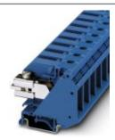
N disconnect terminal block, Special and hybrid connection, Cross section: 0.75 mm² - 35 mm², AWG: 18 - 2, Width: 15 mm, Color: blue, Mounting type: NS 35/7,5, NS 35/15, NS 32
