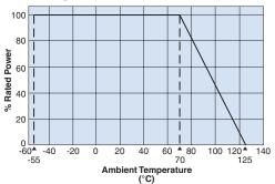
power rating shall be derated in accordance with the above derating curve.
