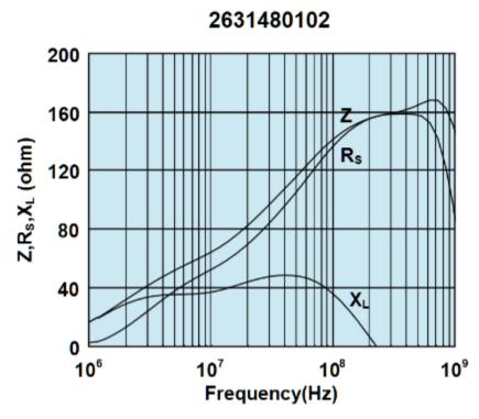
Impedance, reactance, and resistance vs. frequency.
