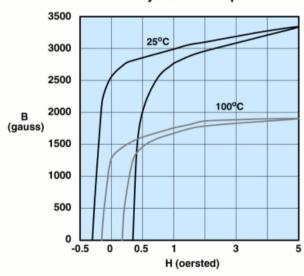
Measured on a 17/10/6mm toroid at 10kHz.
