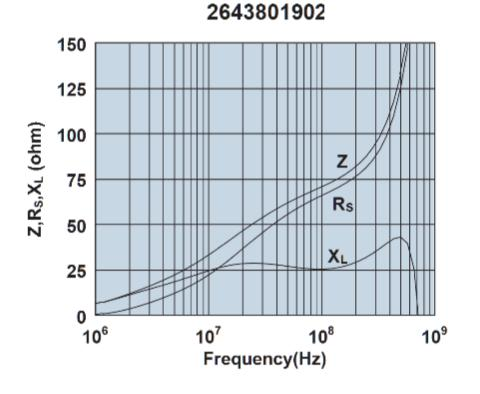
Impedance, reactance, and resistance vs. frequency.
