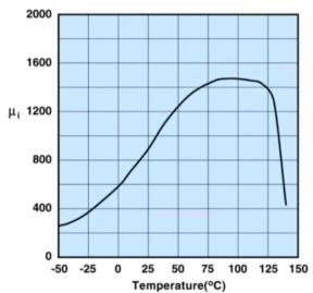
Measured on a 17/10/6mm toroid at 100kHz.
