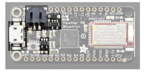
The above shows the Micro USB jack (left), Lipoly JST jack (top left), as well as the 3.3V regulator and changeover diode (just to the right of the JST jack) and the Lipoly charging circuitry (to the right of the Reset button). There's also a **CHG** LED, which will light up while the battery is charging. This LED might also flicker if the battery is not connected.
