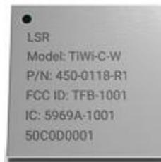
The module includes the necessary PHY, MAC, and network layers to support WLAN applications on the integrated applications processor, or through a simple host interface.
