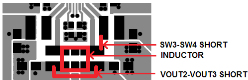
Figure 6. Combined 3A Regulator Inductor Placement and Connections
