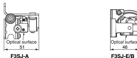
**Replacement using intermediate brackets**
