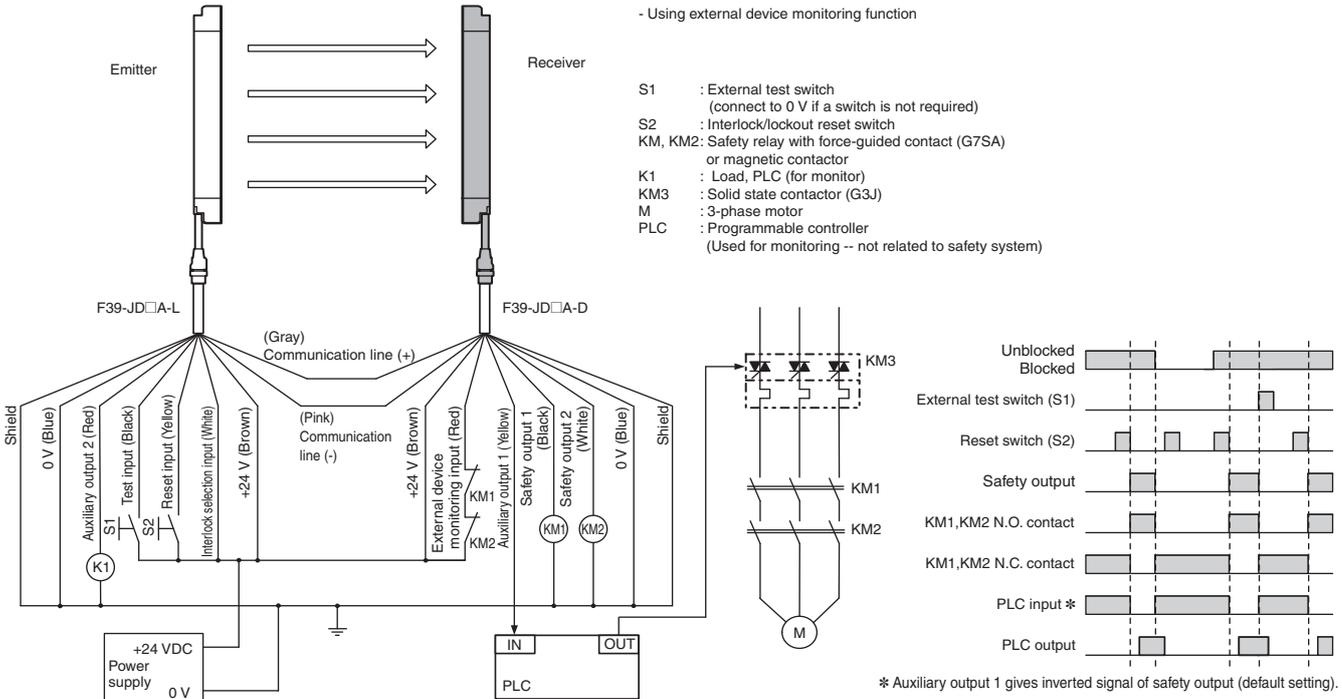
Wiring for connection with a controller F3SP-B1P [PNP Output]
