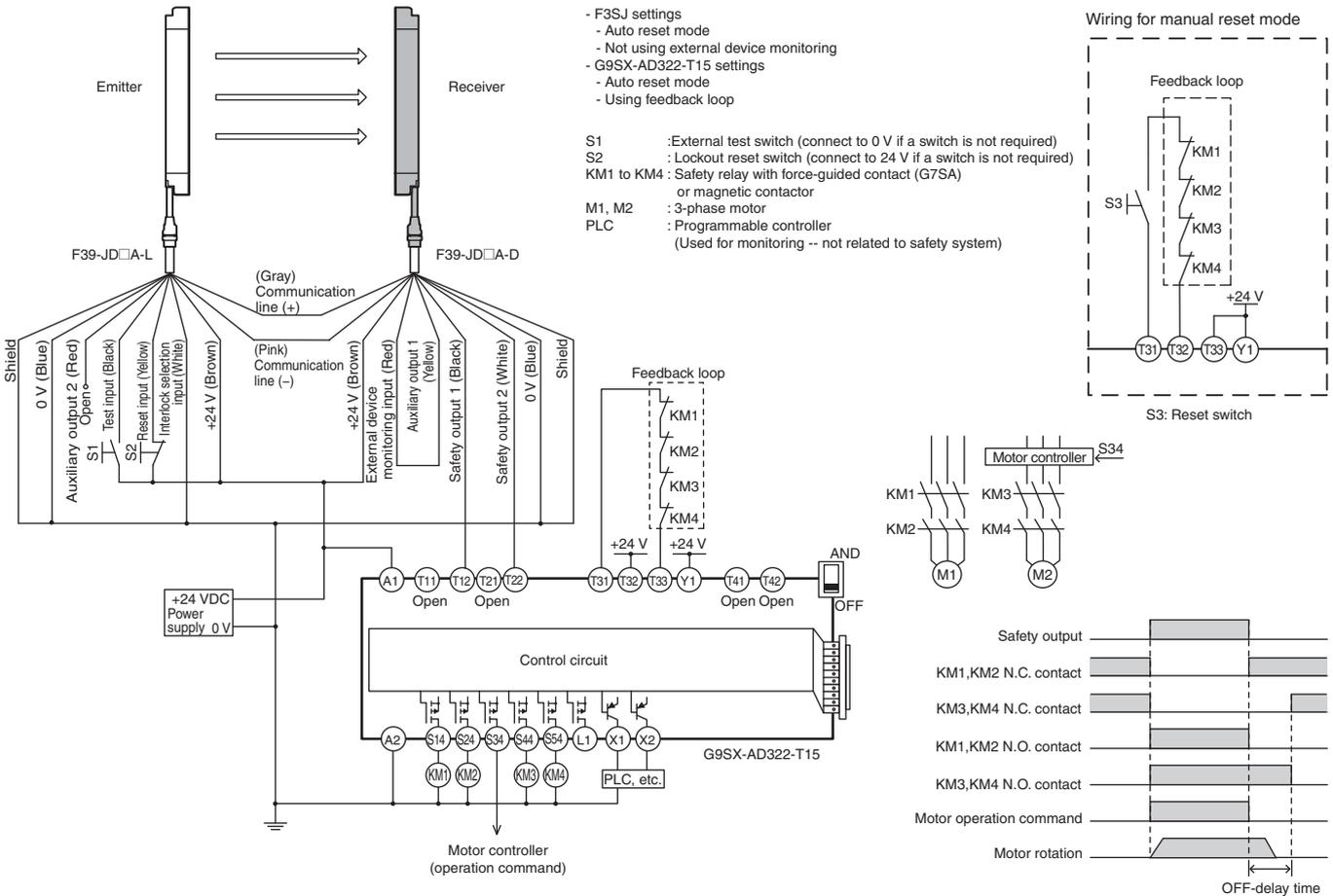
Wiring for single F3SJ-A application [NPN Output]
