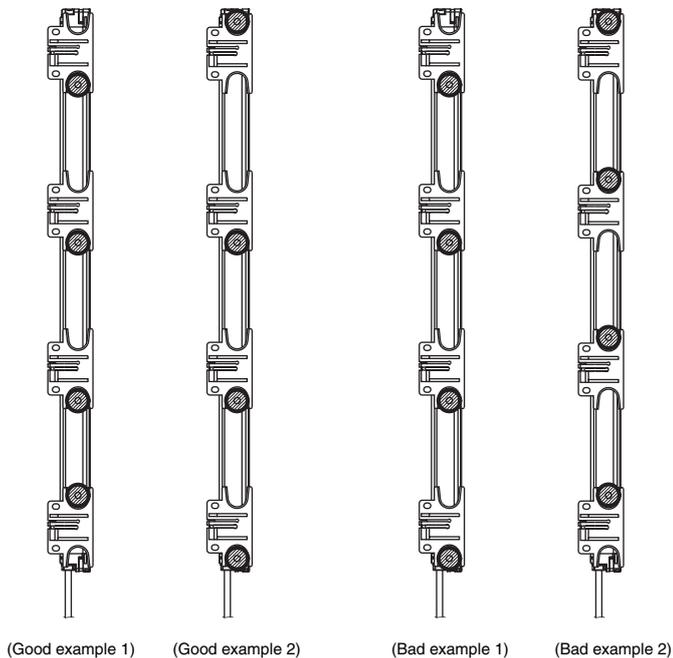
Mount Quick Mount M6 Brackets (or Quick Mount M8 Brackets) according to the mounting positions of the emitter and receiver. The positions of Intermediate Brackets mounted to the emitter and receiver must be aligned with each other.
