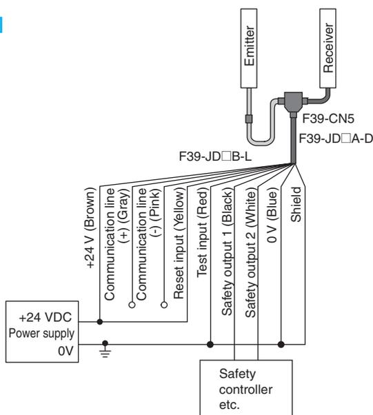
Controllers connectable with PNP output F3SJ series
