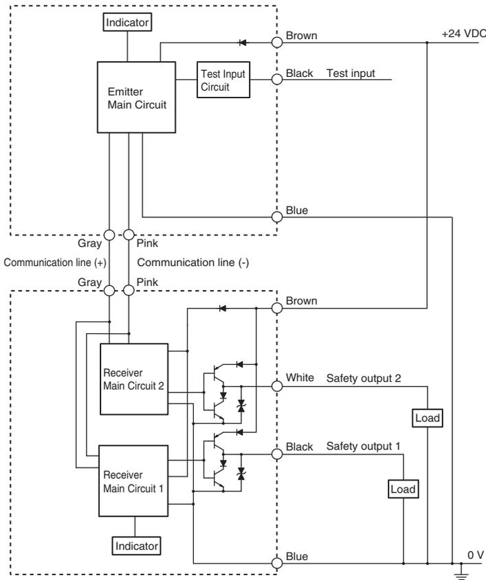
**Input circuit diagram by function**
