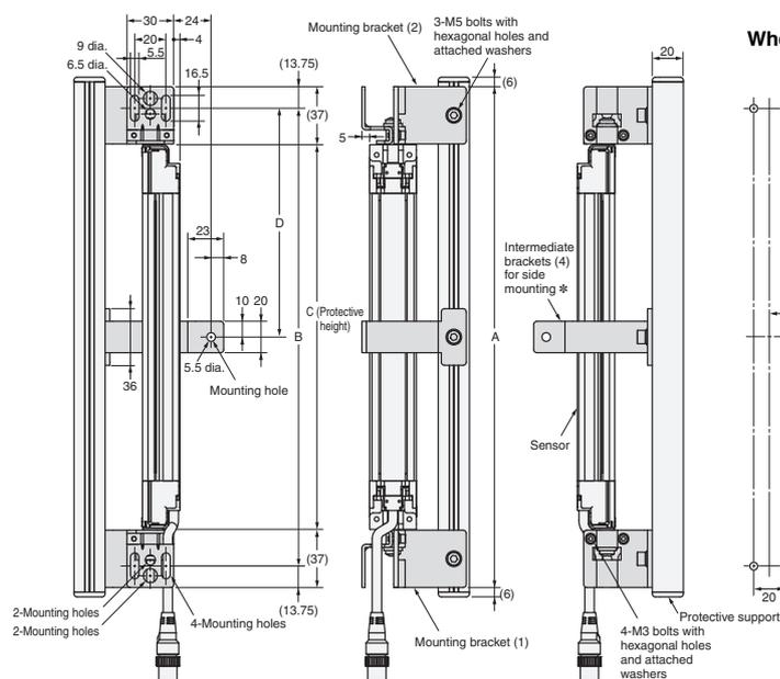
\*The four intermediate brackets (F39-PJ-MS) for side mounting are not provided.
