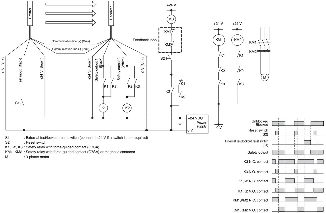
**Wiring to connect a F3SJ-E with a controller G9SP [PNP Output]**
