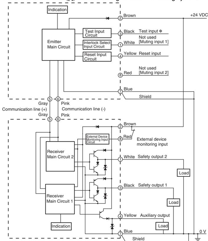
\* The light emission stops when applying voltage of Vs-3 V to Vs to the test input line.
