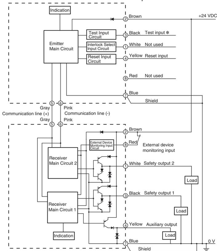
\* The light emission stops when opening the test input line or applying voltage of 0 V to 1/2 Vs to the test input line.
