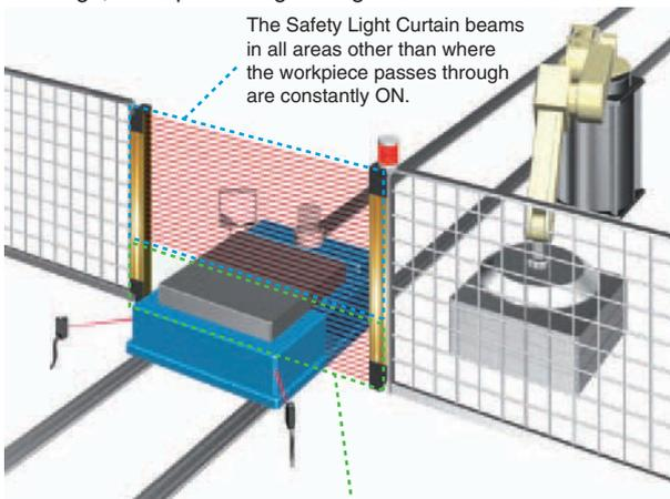
The Safety Light Curtain beams in all areas other than where the workpiece passes through are constantly ON.
