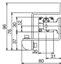
Side mounting (using M8 screws)
