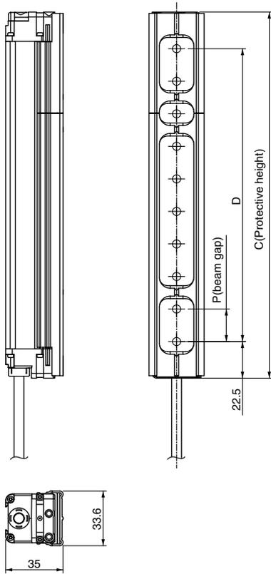
**Note:** For information on dimensions with brackets mounted, refer to the User's Manual of the F3SJ-B□□□□P25-02TS (SCHG-736). Brackets used are common to other F3SJ-E/B series.
