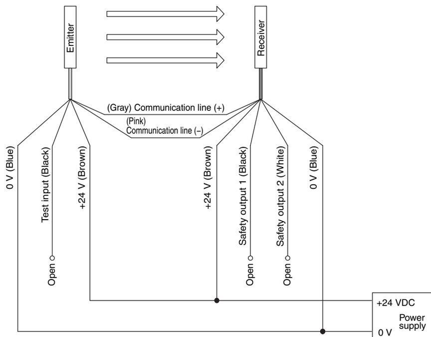
**Note:** This circuit diagram is used for operation check. For an actual circuit example, refer to page 23.
