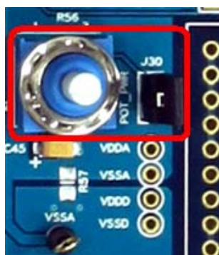
Figure 4-7 CY8CKIT-030 PSoC 3 DVK Potentiometer Power
