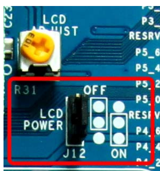
Figure 4-4 CY8CKIT-001 PSoC DVK LCD Power Jumper
