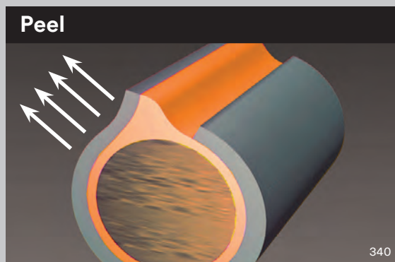
Peel Peel is concentrated along a thin line at the edge of the bond where one substrate is flexible.
