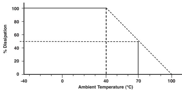
Dissipation as a function of temperature.
