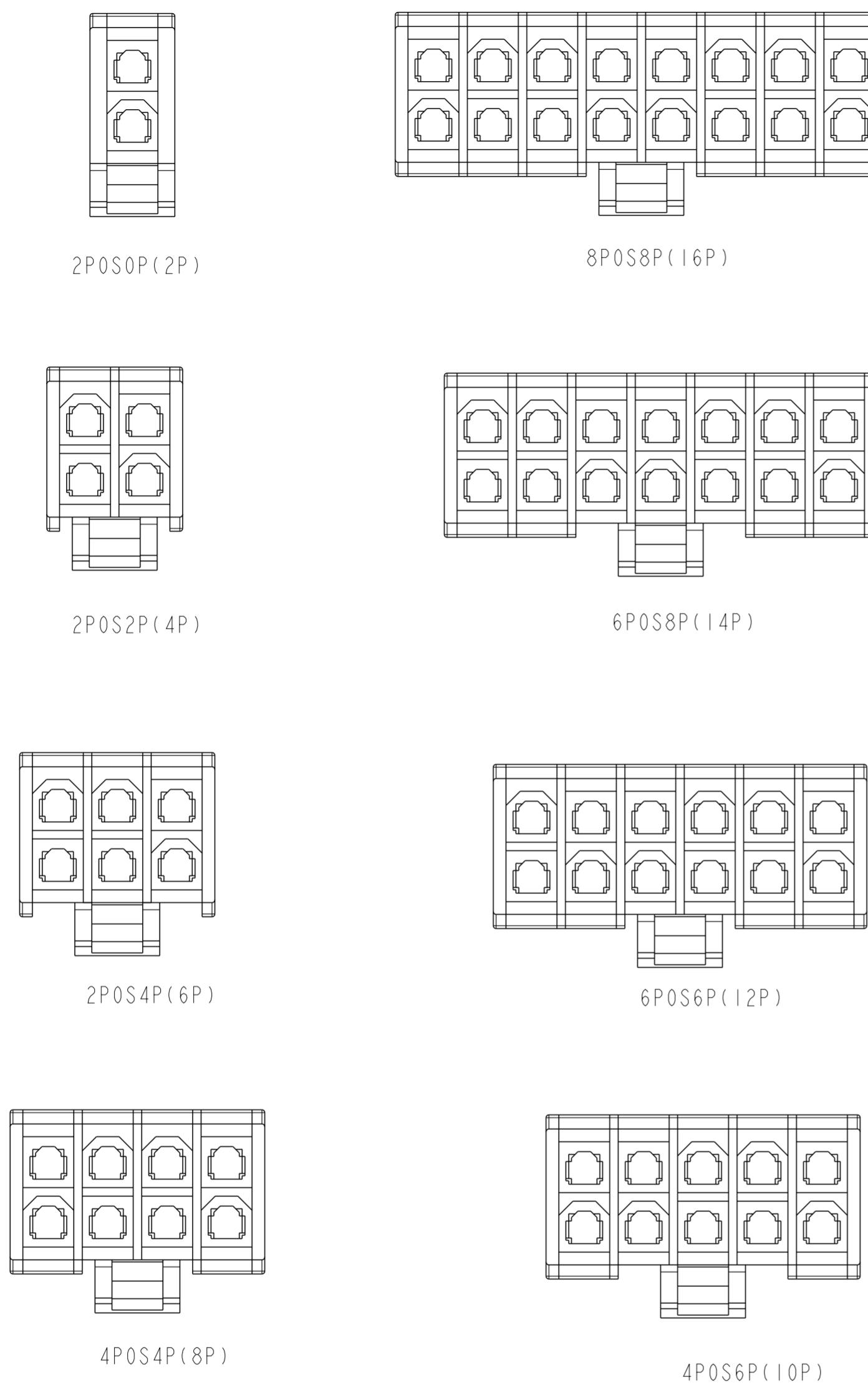
POWER PIN LAYOUT (WITH OR WITHOUT SIGNAL PINS)
