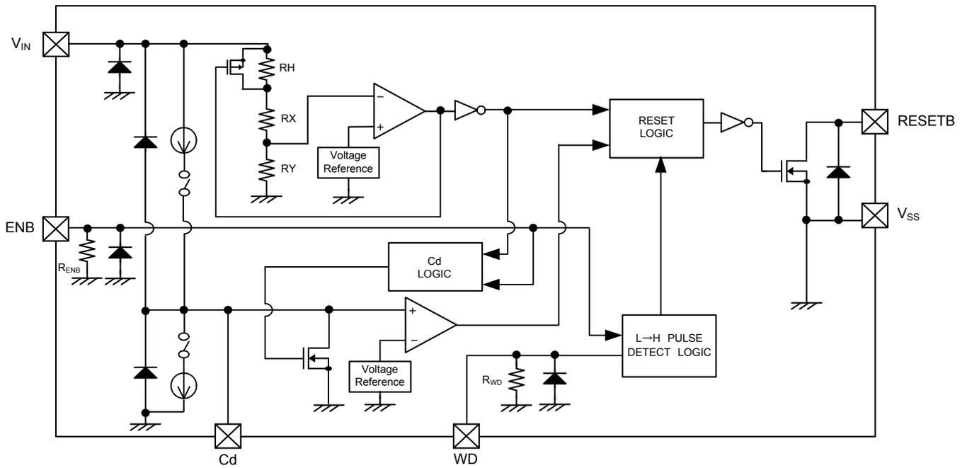
\* Diodes inside the circuit are an ESD protection diode and a parasitic diode.
