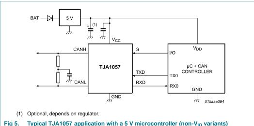
Typical TJA1057 application with a 5 V microcontroller (non-V<sub>IO</sub> variants)
