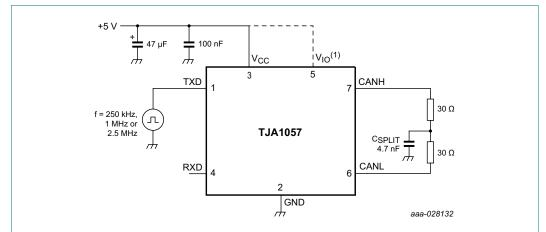
(1) The  $V_{IO}$  pin is internally connected to pin  $V_{CC}$  in the non- $V_{IO}$  product variants TJA1057(G)T(K).
