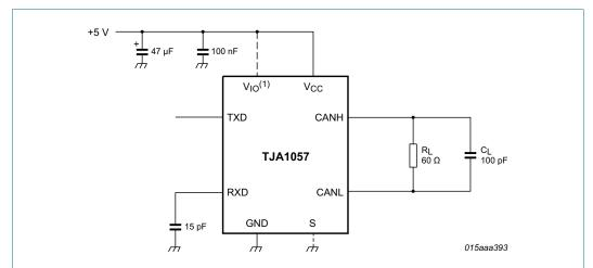
(1) The  $V_{IO}$  pin is internally connected to pin  $V_{CC}$  in the non- $V_{IO}$  product variants TJA1057(G)T(K).
