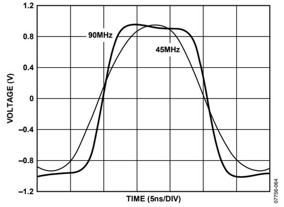
Figure 57. Large Signal Transient Response (Low-Pass Filter)
