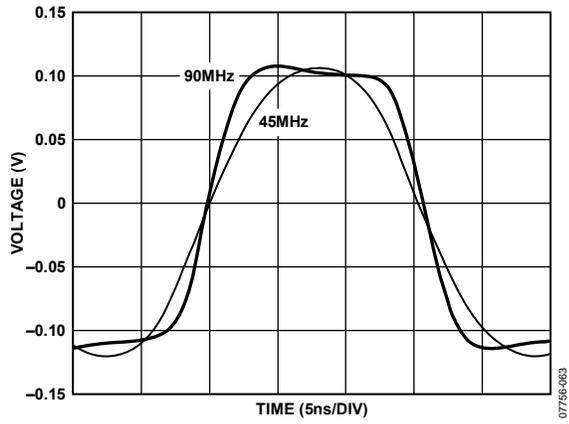
Figure 56. Small Signal Transient Response (Low-Pass Filter)
