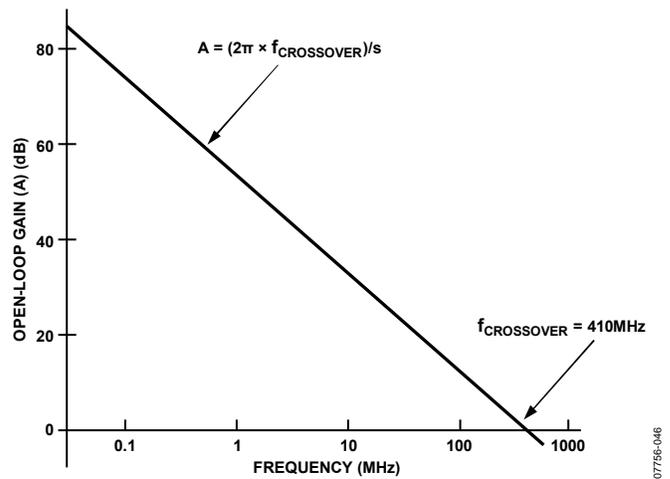
Figure 43. Open-Loop Gain vs. Frequency and Basic Connections
