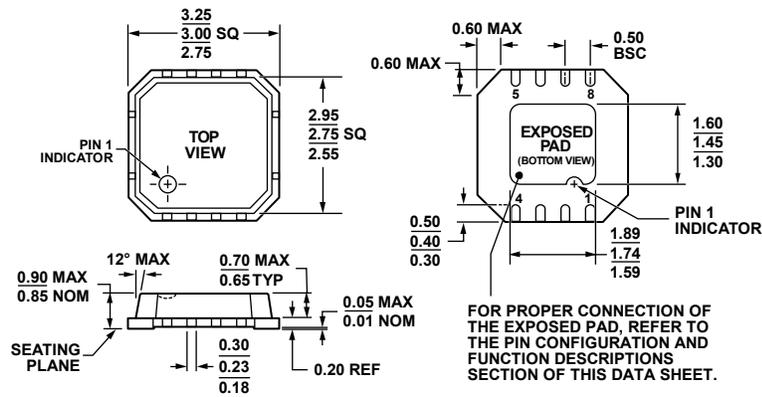
Figure 58. 8-Lead Lead Frame Chip Scale Package [LFCSP\_VD]
