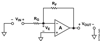
Figure 42. Inverting Configuration
