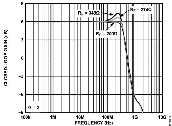
Figure 13. Small Signal Frequency Response for Various  $R_F$
