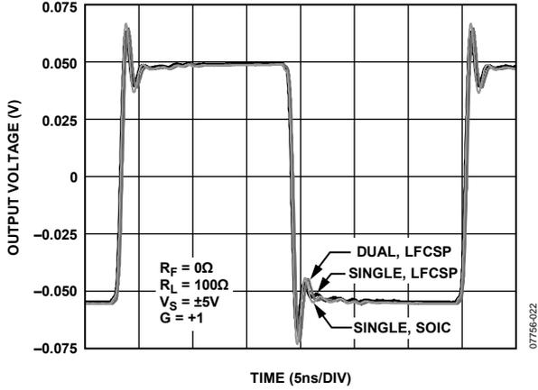
Figure 21. Small Signal Transient Response vs. Package
