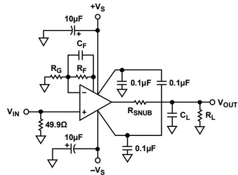
Figure 45.  $R_{SNUB}$  or  $C_F$  Used to Reduce Peaking
