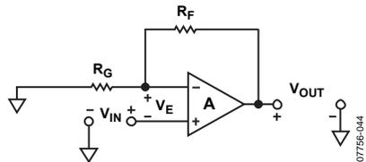
Figure 41. Noninverting Configuration
