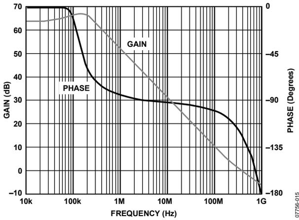
Figure 33. Open-Loop Gain and Phase vs. Frequency
