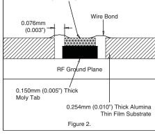
General Handling: Handle the chip along the edges with a vacuum collet or with a sharp pair of bent tweezers. The surface of the chip may have fragile air bridges and should not be touched with vacuum collet, tweezers, or fingers.
