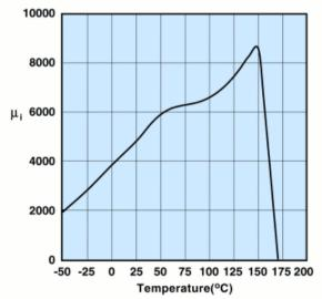
Measured on a 17/10/6mm toroid at 10kHz.
