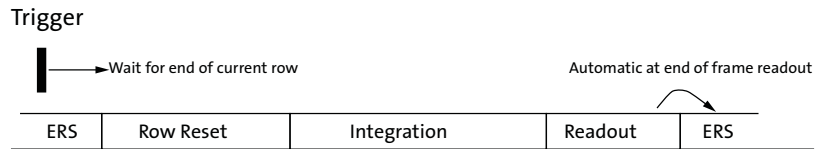
Figure 16: Entering and Leaving a Global Reset Sequence
