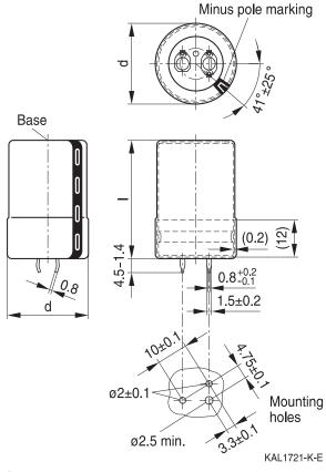
Snap-in terminals, length (6.3 + 1/-1.4) mm. Also available in a shorter version with a length of (4.5 - 1.4) mm. PET insulation cap is positioned under the insulation sleeve. Safety vent on the base or on the case wall.
