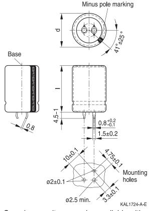
Snap-in capacitors are also available with 3 terminals (length (4.5-1) mm). Insulation is marked with "PET" on the sleeve. Safety vent on the base or on the case wall.
