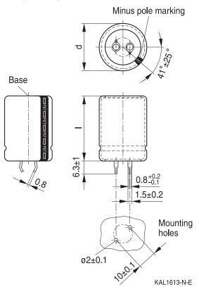
Snap-in terminals, length (6.3  $\pm 1$ ) mm. Also available in a shorter version with a length of (4.5 -1) mm.
