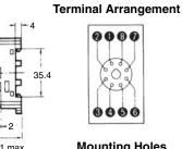
**Mounting Holes** Two, M4 or two 4.5-dia. holes 33±0.2
