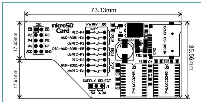
Figure 2: Dimensions of the microSD Card additional board
