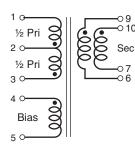
Secondary windings to be connected in parallel on PC board
