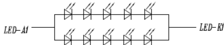
Figure: LED connection of backlight
