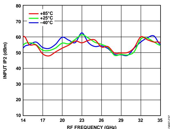
Figure 37. Input IP2 vs. RF Frequency over Various Temperatures,
