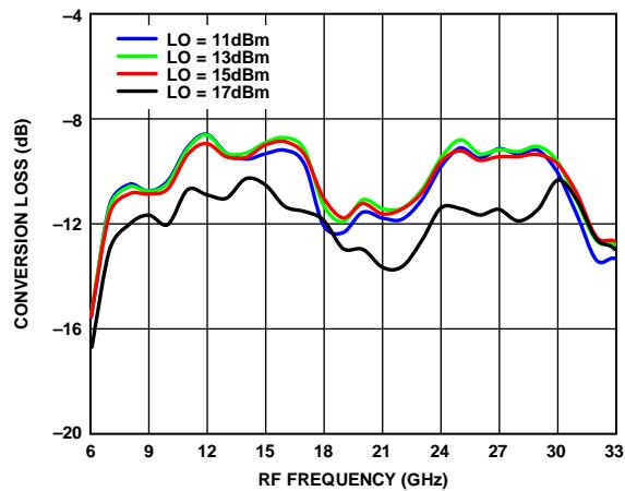
Figure 65. Conversion Loss vs. RF Frequency over LO Drives
