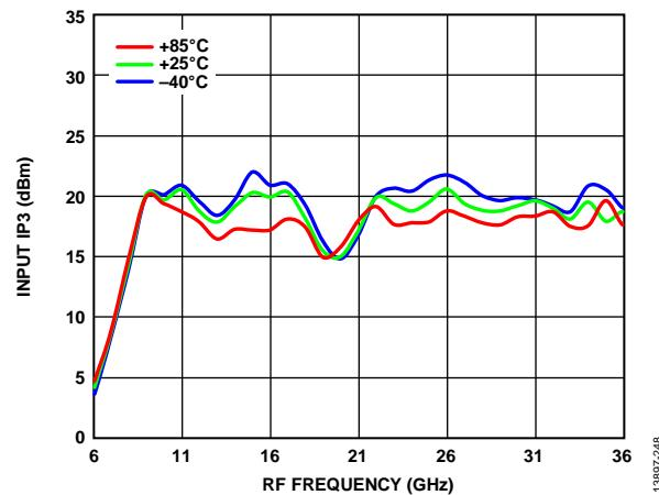
Figure 48. Input IP3 vs. RF Frequency over Various Temperatures,
