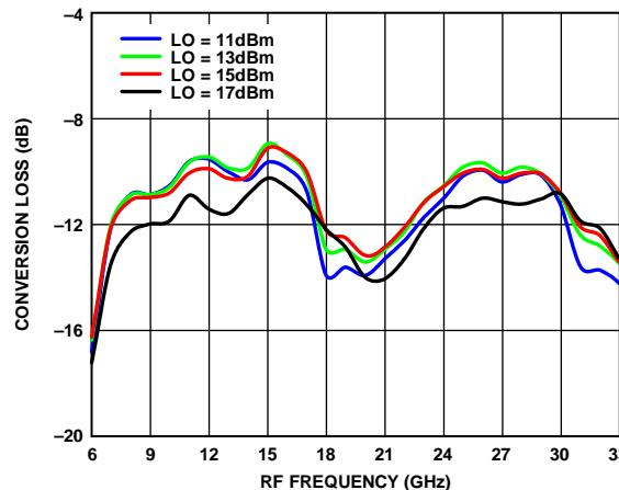
Figure 32. Conversion Loss vs. RF Frequency over Various LO Drives
