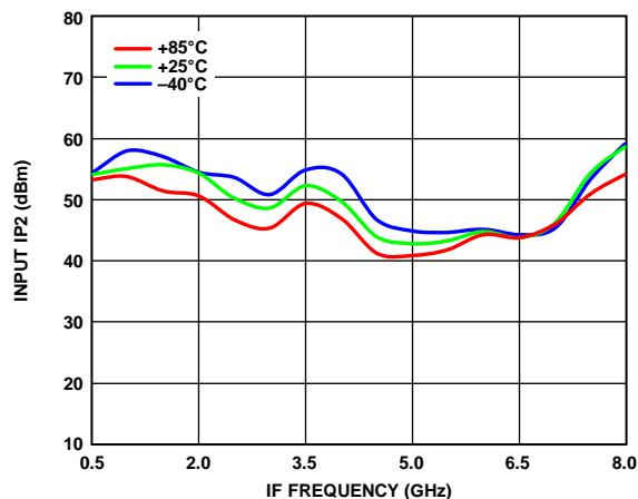
Figure 77. Input IP2 vs. IF Frequency over Various Temperatures,
