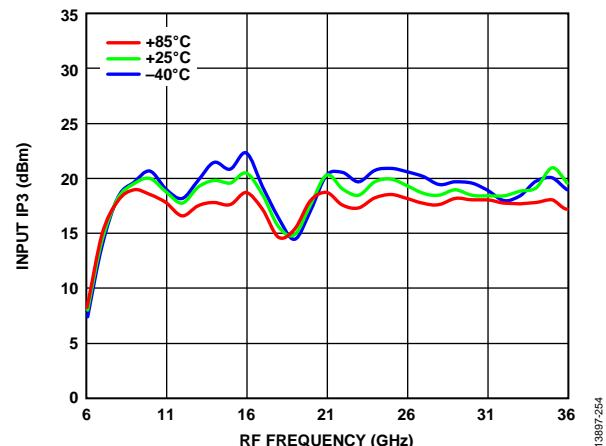
Figure 54. Input IP3 vs. RF Frequency over Various Temperatures,
