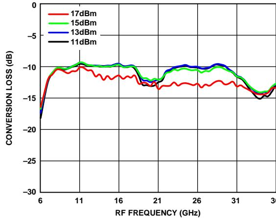
Figure 56. Conversion Loss vs. RF Frequency over LO Drives
