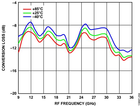
Figure 59. Conversion Loss vs. RF Frequency over Various Temperatures,
