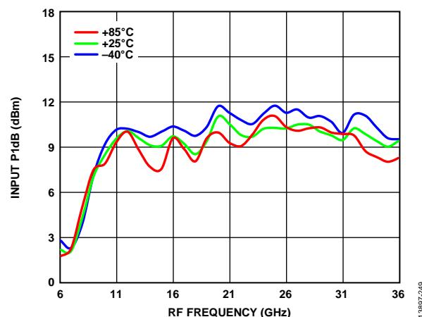
Figure 49. Input P1dB vs. RF Frequency over Various Temperatures,
