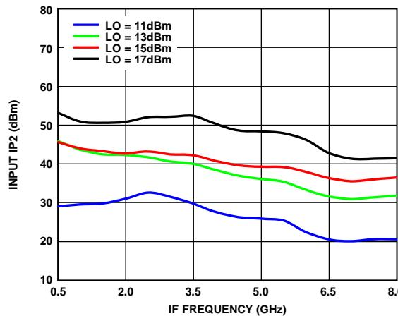
Figure 86. Input IP2 vs. IF Frequency over Various LO Drives
