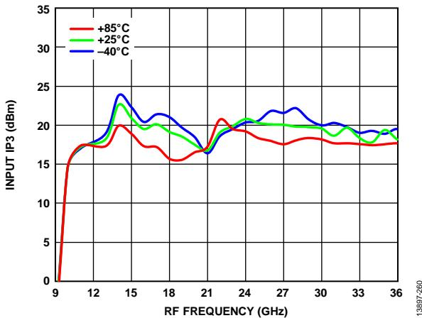
Figure 60. Input IP3 vs. RF Frequency over Various Temperatures,
