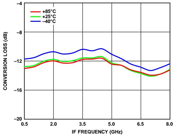
Figure 81. Conversion Loss vs. IF Frequency over Various Temperatures,
