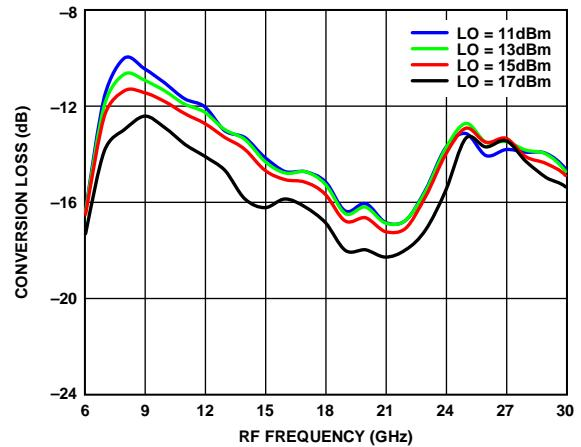
Figure 73. Conversion Loss vs. RF Frequency over LO Drives
