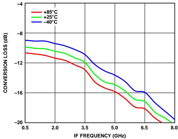
Figure 75. Conversion Loss vs. IF Frequency over Various Temperatures,
