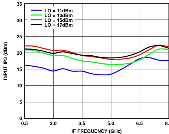
Figure 85. Input IP3 vs. IF Frequency over Various LO Drives
