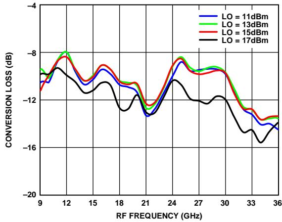
Figure 61. Conversion Loss vs. RF Frequency over LO Drives
