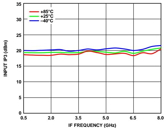
Figure 76. Input IP3 vs. IF Frequency over Various Temperatures,
