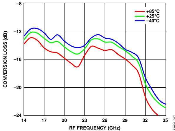
Figure 67. Conversion Loss vs. RF Frequency over Various Temperatures,
