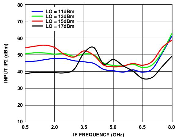
Figure 80. Input IP2 vs. IF Frequency over Various LO Drives
