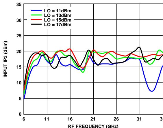
Figure 57. Input IP3 vs. RF Frequency over Various LO Drives
