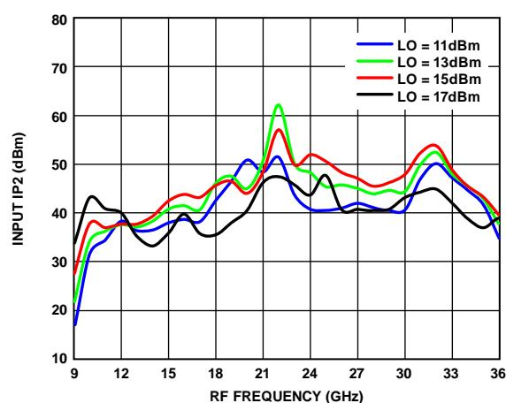
Figure 28. Input IP2 vs. RF Frequency over Various LO Drives
