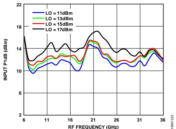
Figure 22. Input P<sub>1dB</sub> vs. RF Frequency over Various LO Drives
