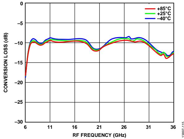
Figure 47. Conversion Loss vs. RF Frequency over Various Temperatures,
