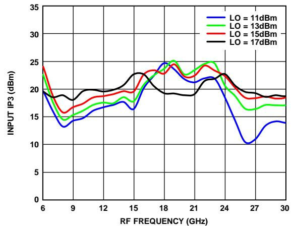
Figure 74. Input IP3 vs. RF Frequency over Various LO Drives
