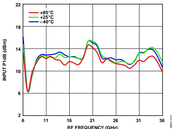
Figure 13. Input P<sub>1dB</sub> vs. RF Frequency over Various Temperatures,
