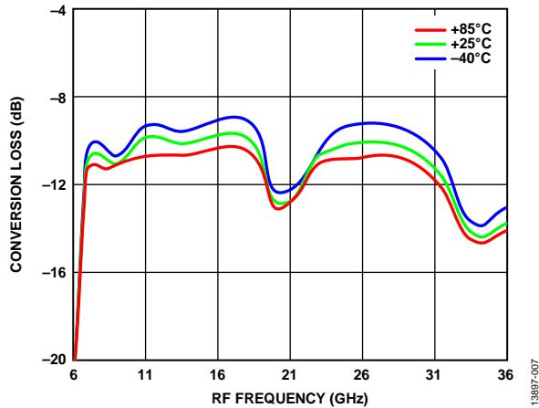
Figure 15. Conversion Loss vs. RF Frequency over Various Temperatures,
