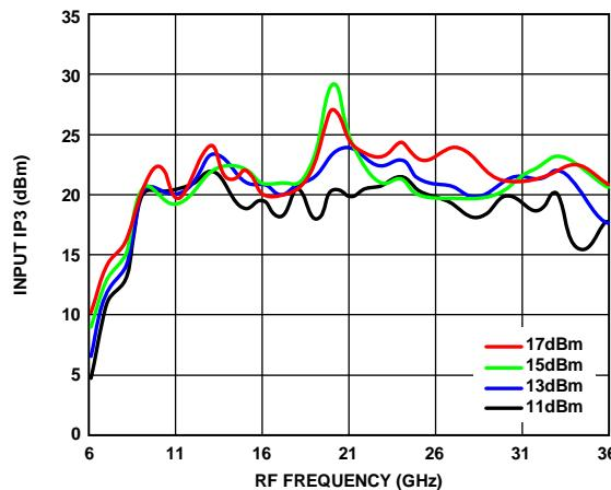
Figure 19. Input IP3 vs. RF Frequency over Various LO Drives
