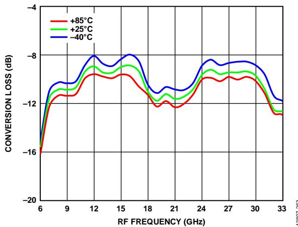
Figure 63. Conversion Loss vs. RF Frequency over Various Temperatures,
