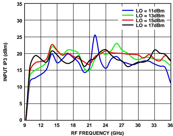
Figure 62. Input IP3 vs. RF Frequency over Various LO Drives
