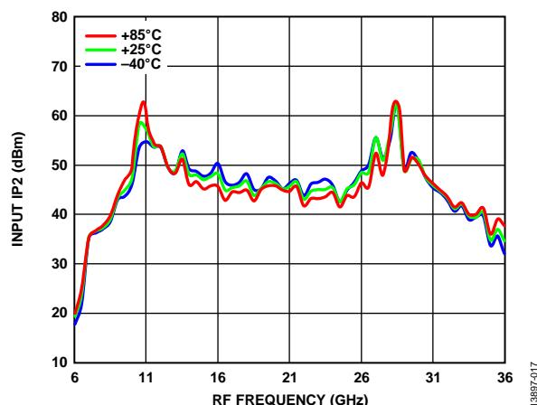
Figure 17. Input IP2 vs. RF Frequency over Various Temperatures,
