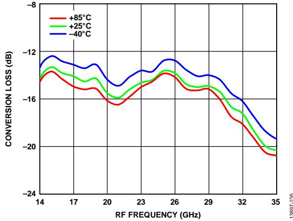
Figure 35. Conversion Loss vs. RF Frequency over Various Temperatures,
