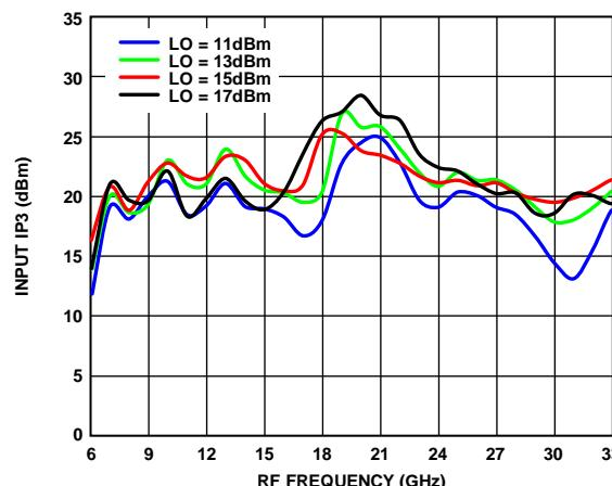
Figure 33. Input IP3 vs. RF Frequency over Various LO Drives
