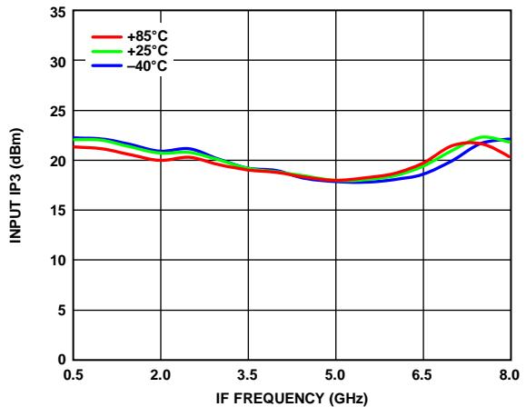
Figure 82. Input IP3 vs. IF Frequency over Various Temperatures,
