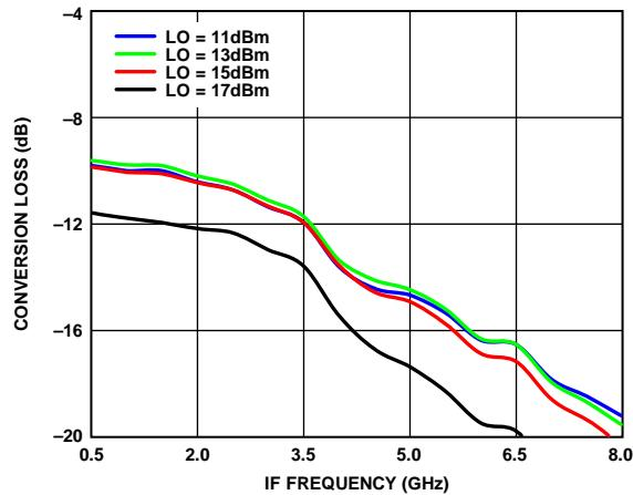
Figure 78. Conversion Loss vs. IF Frequency over Various LO Drives
