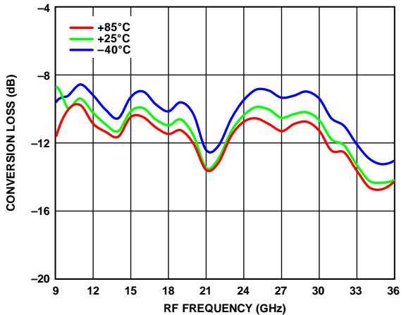
Figure 23. Conversion Loss vs. RF Frequency over Various Temperatures,
