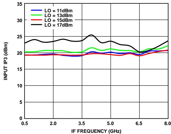
Figure 79. Input IP3 vs. IF Frequency over Various LO Drives
