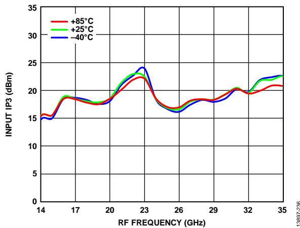
Figure 36. Input IP3 vs. RF Frequency over Various Temperatures,
