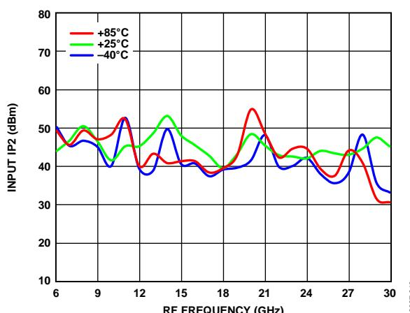
Figure 43. Input IP2 vs. RF Frequency over Various Temperatures,
