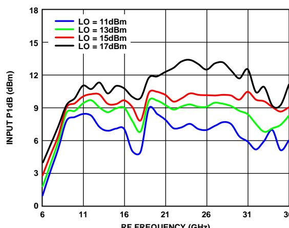
Figure 58. Input P1dB vs. RF Frequency over Various LO Drives
