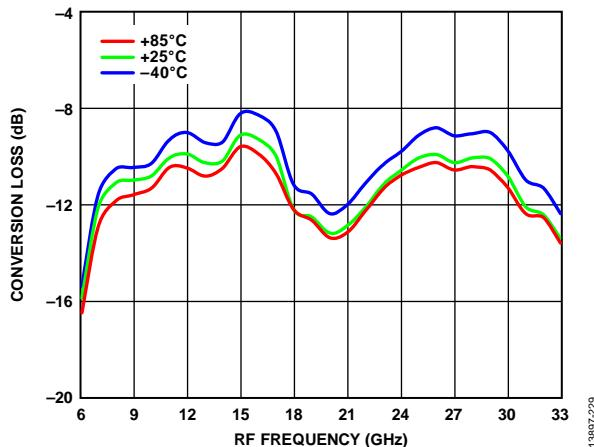
Figure 29. Conversion Loss vs. RF Frequency over Various Temperatures,
