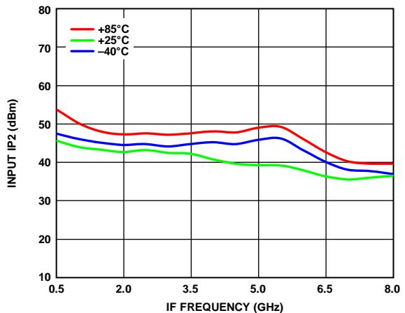
Figure 83. Input IP2 vs. IF Frequency over Various Temperatures,
