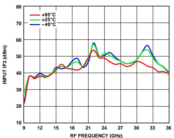
Figure 25. Input IP2 vs. RF Frequency over Various Temperatures,
