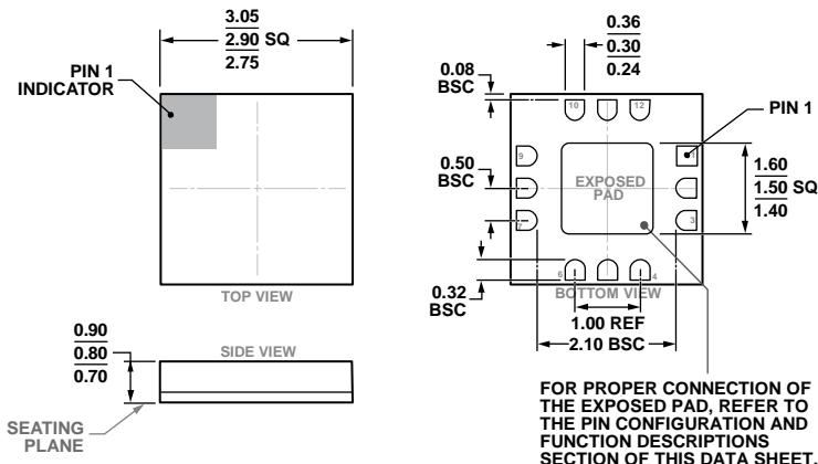
Figure 98. 12-Terminal Ceramic Leadless Chip Carrier [LCC]
