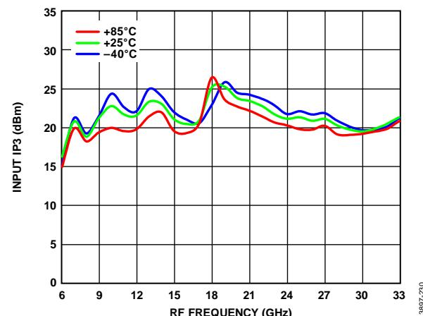
Figure 30. Input IP3 vs. RF Frequency over Various Temperatures,
