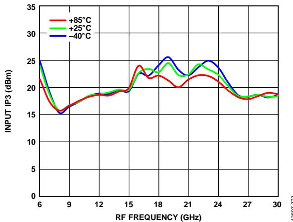
Figure 72. Input IP3 vs. RF Frequency over Various Temperatures,
