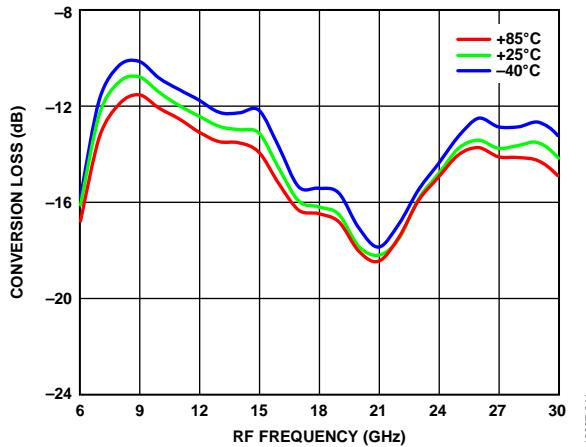
Figure 41. Conversion Loss vs. RF Frequency over Various Temperatures,
