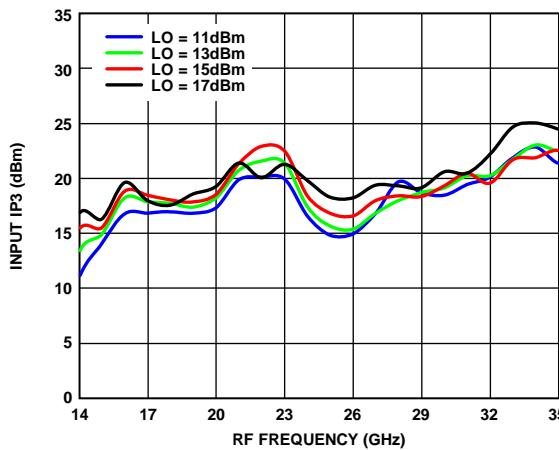
Figure 39. Input IP3 vs. RF Frequency over Various LO Drives
