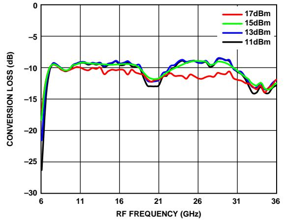
Figure 50. Conversion Loss vs. RF Frequency over LO Drives
