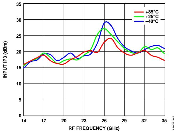
Figure 68. Input IP3 vs. RF Frequency over Various Temperatures,
