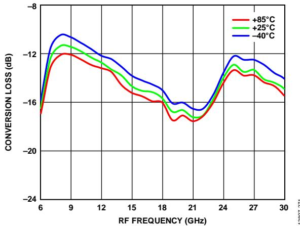
Figure 71. Conversion Loss vs. RF Frequency over Various Temperatures,
