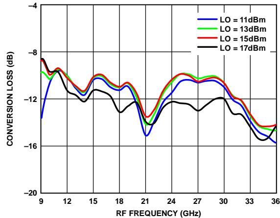
Figure 26. Conversion Loss vs. RF Frequency over Various LO Drives
