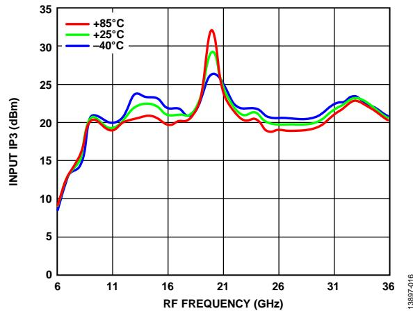
Figure 16. Input IP3 vs. RF Frequency over Various Temperatures,
