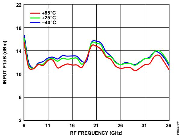
Figure 21. Input P<sub>1dB</sub> vs. RF Frequency over Various Temperatures,
