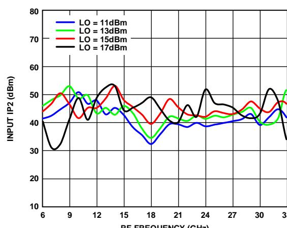
Figure 34. Input IP2 vs. RF Frequency over Various LO Drives
