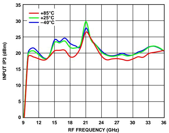
Figure 24. Input IP3 vs. RF Frequency over Various Temperatures,
