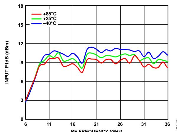
Figure 55. Input P1dB vs. RF Frequency over Various Temperatures,
