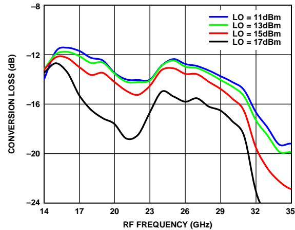
Figure 69. Conversion Loss vs. RF Frequency over LO Drives
