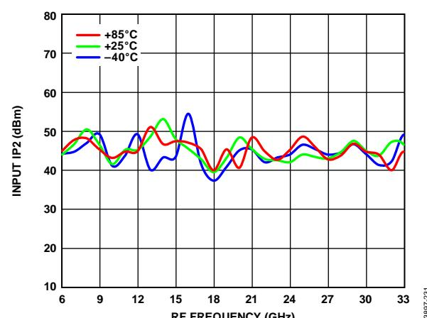
Figure 31. Input IP2 vs. RF Frequency over Various Temperatures,
