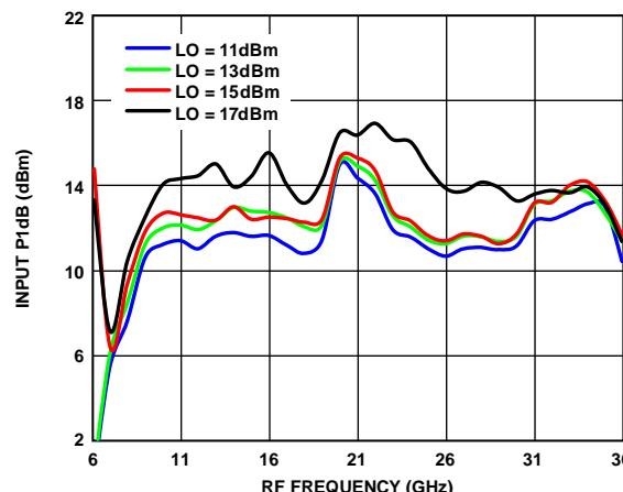
Figure 14. Input P<sub>1dB</sub> vs. RF Frequency over Various LO Drives
