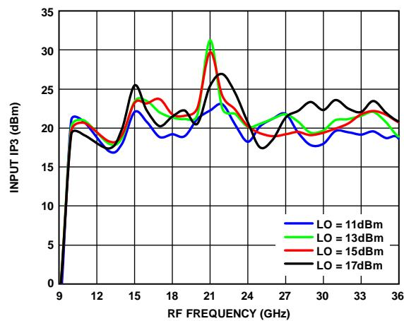
Figure 27. Input IP3 vs. RF Frequency over Various LO Drives
