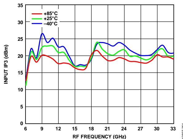
Figure 64. Input IP3 vs. RF Frequency over Various Temperatures,
