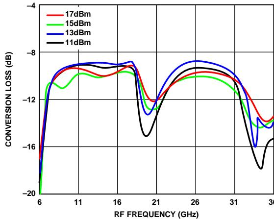
Figure 18. Conversion Loss vs. RF Frequency over LO Drives
