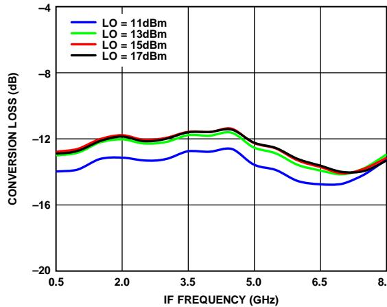
Figure 84. Conversion Loss vs. IF Frequency over Various LO Drives
