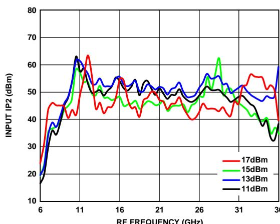
Figure 20. Input IP2 vs. RF Frequency over Various LO Drives
