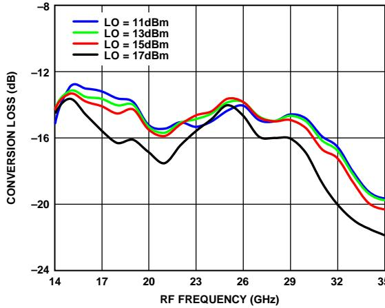
Figure 38. Conversion Loss vs. RF Frequency over Various LO Drives
