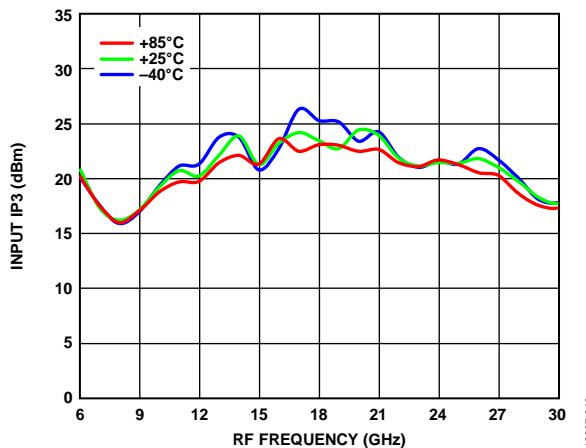
Figure 42. Input IP3 vs. RF Frequency over Various Temperatures,
