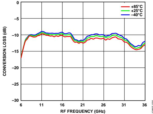
Figure 53. Conversion Loss vs. RF Frequency over Various Temperatures,
