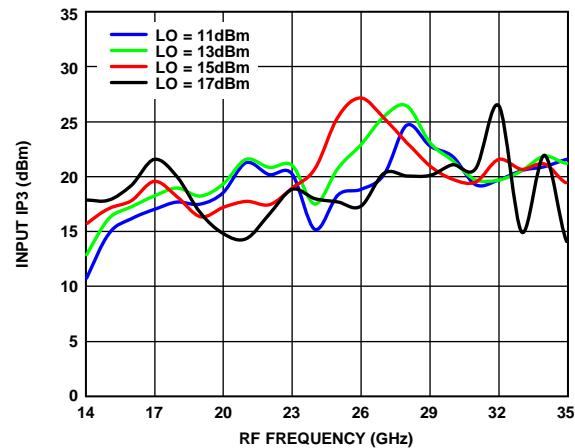
Figure 70. Input IP3 vs. RF Frequency over Various LO Drives
