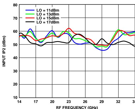
Figure 40. Input IP2 vs. RF Frequency over Various LO Drives
