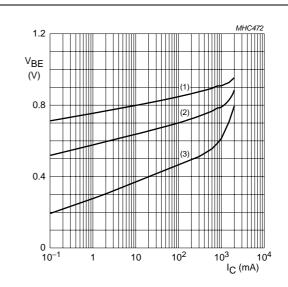
**TR1 (NPN);**  $V_{CE} = 5 \text{ V}.$
