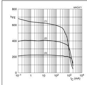
**TR1 (NPN);**  $V_{CE} = 5 \text{ V}.$
