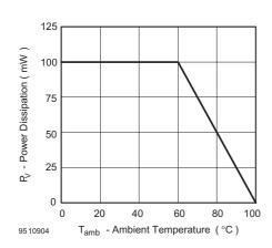
Figure 1. Power Dissipation vs. Ambient Temperature
