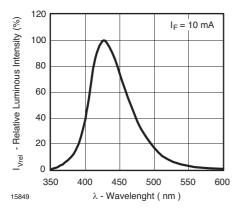
Figure 7. Relative Intensity vs. Wavelength
