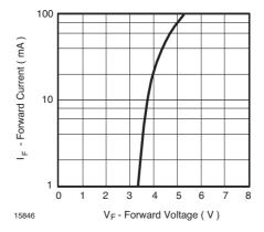
Figure 4. Forward Current vs. Forward Voltage
