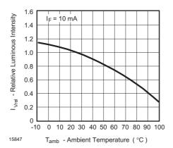
Figure 5. Rel. Luminous Flux vs. Ambient Temperature
