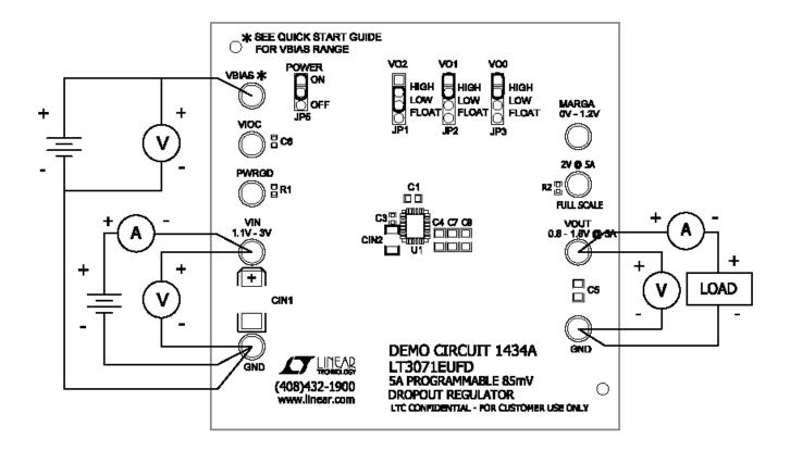
Figure 1. Proper Measurement Equipment Setup
