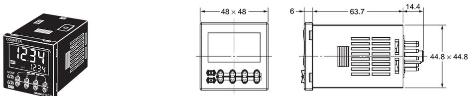
Dimensions with Flush Mounting Adapter
