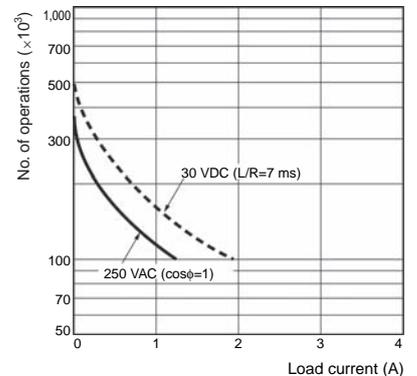
A current of 0.15 A max. can be switched at 125 VDC (cosφ=1) and current of 0.1 A max. can be switched if L/R=7 ms. In both cases, a life of 100,000 operations can be expected.
