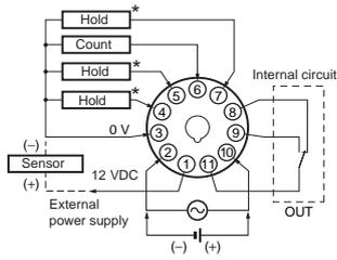
\* The hold function is the same whichever terminal is connected. Terminals are not connected internally, and so do not use them for cross-over wiring.
