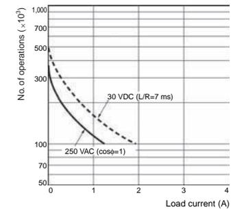
A current of 0.15 A max. can be switched at 125 VDC (cosφ=1) (Life expectancy: 100,000 operations)
