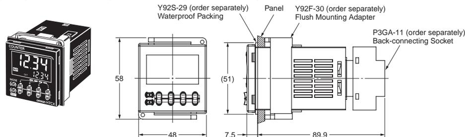
Dimensions with Front Connecting Socket
