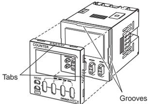
The Front Panel is attached to the Counter/Tachometer with tabs in four locations. To remove the Front Panel, open the tabs and pull the Front Panel forward. To attach the Front Panel, press it onto the Counter/Tachometer so that all four tabs lodge into the grooves on the body of the Counter/Tachometer.
