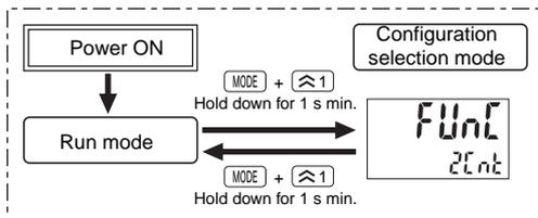
Switch from 2Cnt (2-stage preset counter mode) to tARd (tachometer mode) using the Key.
