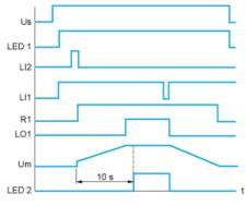
Us : Power supply voltage LED Green LED 1 : LI2, Logic inputs LI1 : R1 : Relay output LO1 :Logic output Um :Motor voltage
