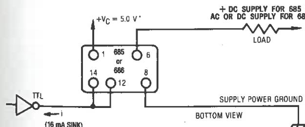
FIGURE 2: FOUR TERMINAL (TTL) USE-SEE NOTE 2
