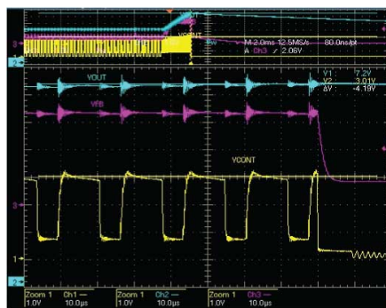
Figure 38. Output voltage ripple at 230 V IN_AC no load
