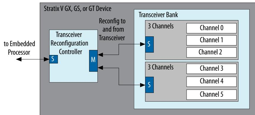
The transceiver PHY IP cores create a separate reconfiguration interface for each channel and each TX PLL. Each transceiver PHY IP core reports the number of reconfiguration interfaces it requires in the message pane of its GUI. You must take note of this number so that you can enter it as a parameter in the Transceiver Reconfiguration Controller.
