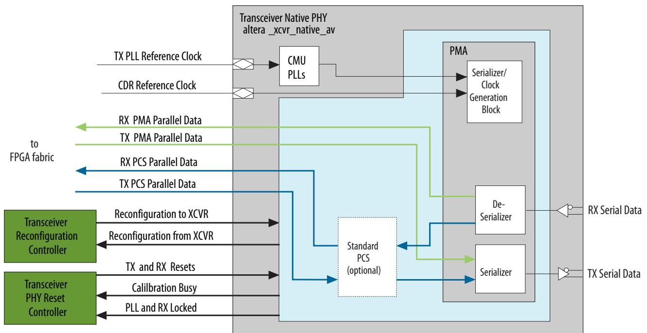
In a typical design, the separately instantiated Transceiver PHY Reset Controller drives reset signals to Native PHY and receives calibration and locked status signal from the Native PHY. The Native PHY reconfiguration buses connect the external Transceiver Reconfiguration Controller for calibration and dynamic reconfiguration of the channel and PLLs.
