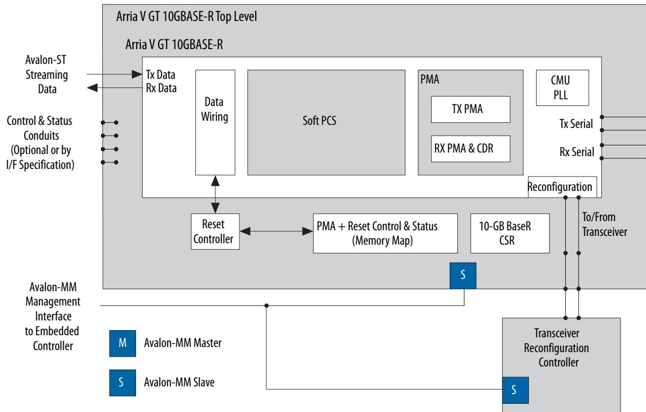
Figure 3-4: 10GBASE-R PHY IP Core In Arria V GZ Devices
