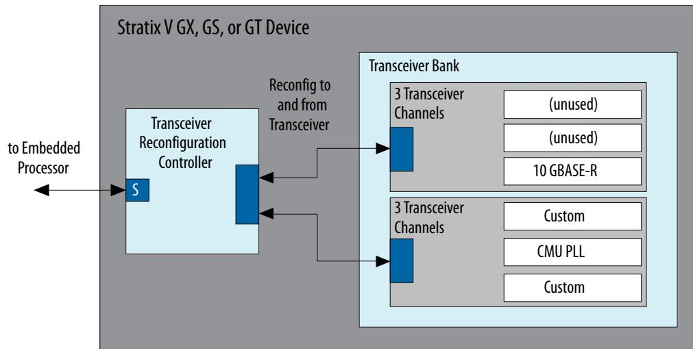
The following figure illustrates incorrect connections between two Transceiver Reconfiguration Controllers and six transceiver channels. Two Transceiver Reconfiguration Controllers cannot access a single reconfiguration interface because there is no arbitration logic to prevent concurrent access. The configuration shown results in a Intel Quartus Prime compilation error.
