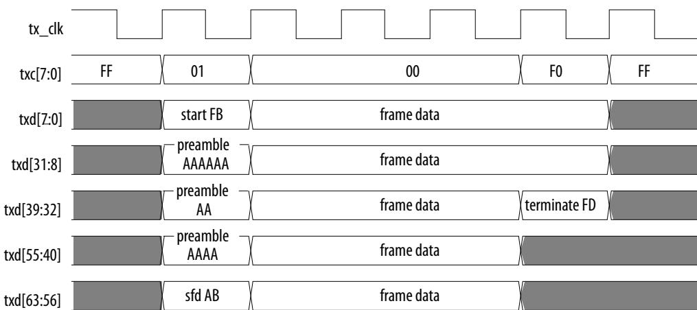
**Figure 7-7: Byte 5 Start of Frame Transmission Example**
