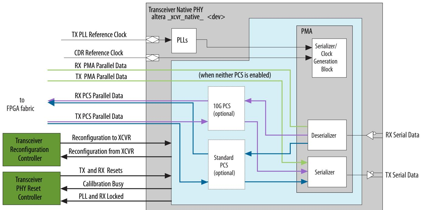
In a typical design, the separately instantiated Transceiver PHY Reset Controller drives reset signals to Native PHY and receives calibration and locked status signal from the Native PHY. The Native PHY reconfiguration buses connect the external Transceiver Reconfiguration Controller for calibration and dynamic reconfiguration of the PLLs.
