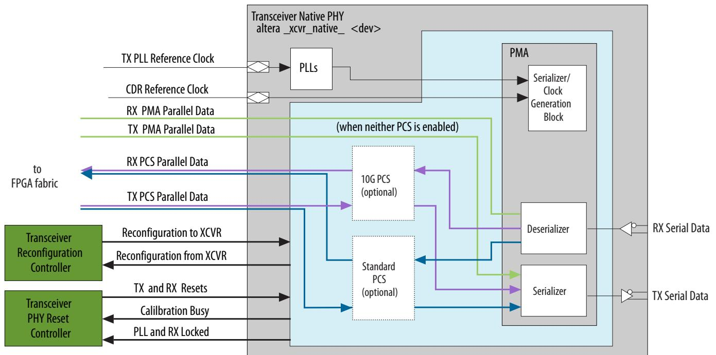
As shown, the Stratix V Native PHY connects to the separately instantiated Transceiver Reconfiguration Controller and Transceiver PHY Reset Controller.
