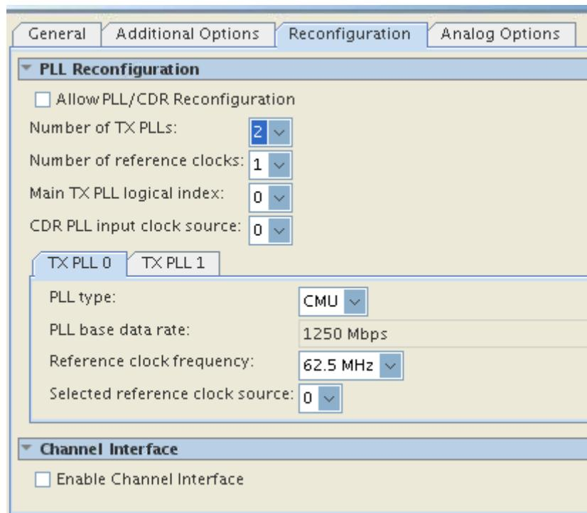
**Figure 17-5: Reconfiguration Tab of Native Transceiver PHYs**
