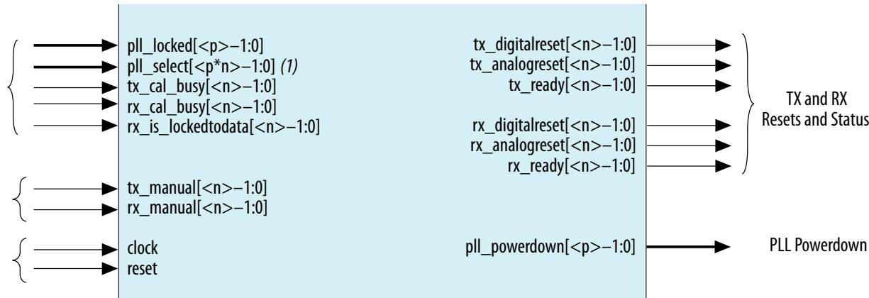
`pll_select` signal width when a single TX reset sequence is used for all channels.
