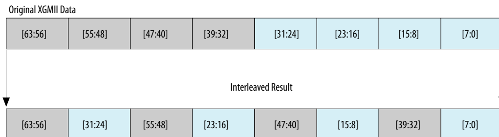
Figure 7-5: Interleaved SDR XGMII Data Mapping
